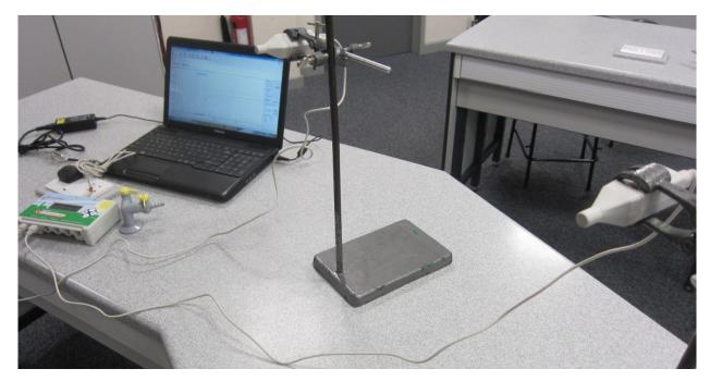
The two sound sensors are mounted on stands and the distance between them can be changed from between 20cm to one metre. They are both connected to a single datalogger and that datalogger is connected via a red tagged USB cable to the laptop.
